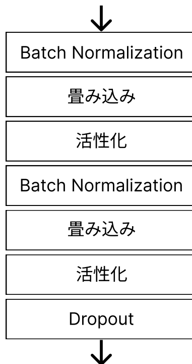
図 3.4: den_con_layer の処理層 (出典 : Dense-UNet: a novel multiphoton in vivo cellular image segmentation model based on a convolutional neural network[22] を参考に作成)
